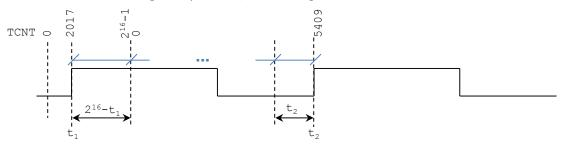
✓ What is the frequency of the signal? E-clock = 24 MHz, Timer Pre-scale Factor = 4.
